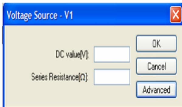
For all other voltage sources, click 'Advanced' and select the type of voltage source and enter the required parameters.
