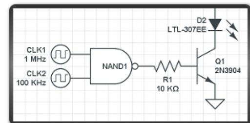
Mixed-mode circuit simulation lets you simulate analog and digital components side-by-side.
