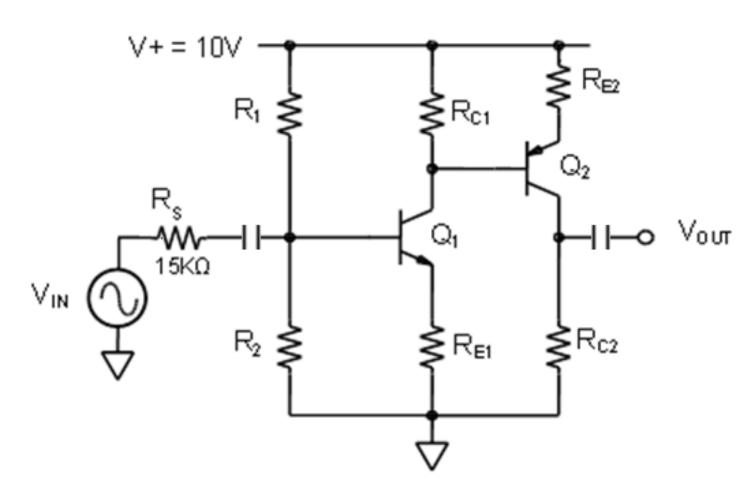
Design a Complementary Pair amplifier stage using 2N3904 and 2N3906 transistor's (β ~ 120, VBE ~ 0.7v). Use a supply voltage of 10 volts, and a source resistance of 15 KΩ. Estimate the DC bias voltages and currents, and compare these with the results of a computer simulation. Determine the small signal voltage gain.
