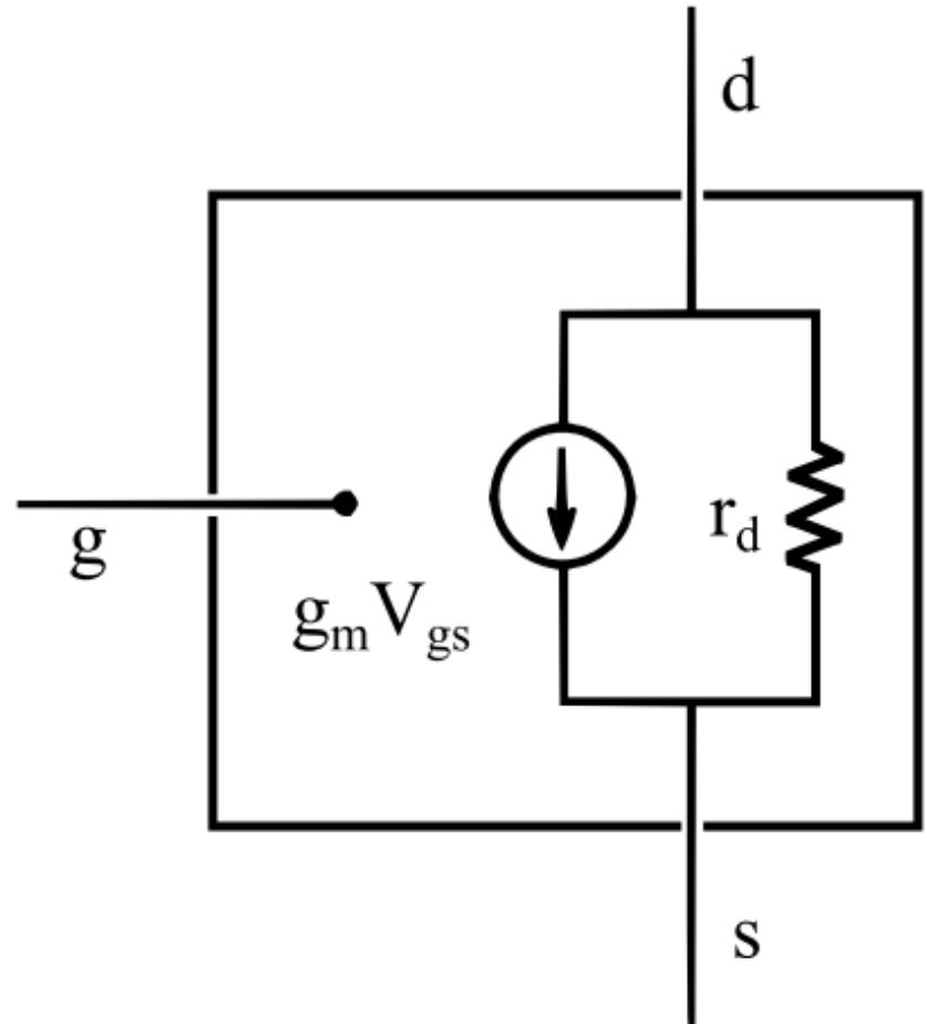
gate – source  $\sim$  open circuit
