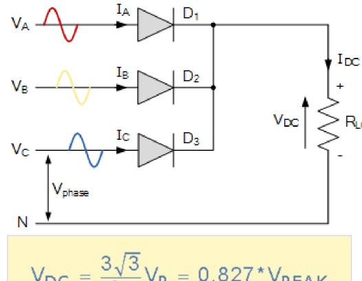
$$V_{DC} = \frac{3\sqrt{3}}{2\pi}V_P = 0.827*V_{PEAK}$$
