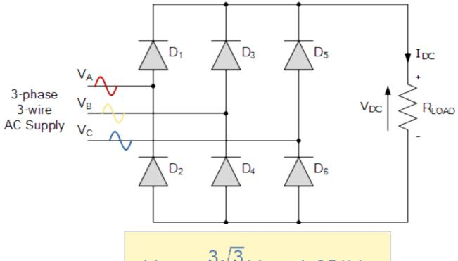
$V_{DC} = \frac{3\sqrt{3}}{\pi}V_{S} = 1.65*V_{S}$
