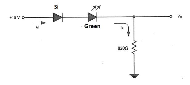
Please find the output voltage  $(V_O)$  and the diode current  $(I_D)$  where  $V_{LED,Green} = 2.2$  Volts.
