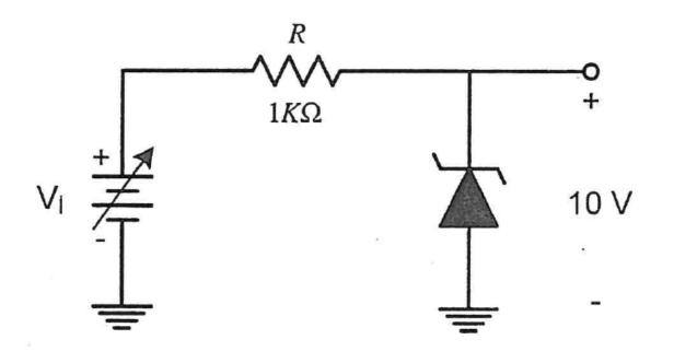
If 10-Volt Zener Diode allows its current 4-40 mA, please find the input voltage range.
