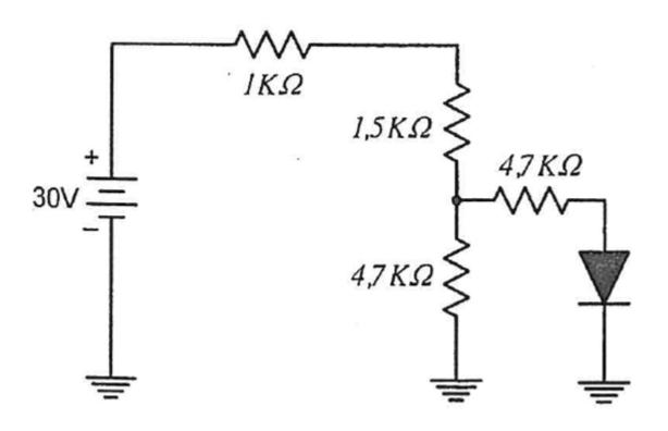
If the diode is Silicon-based, what is the current flown through the diode?
