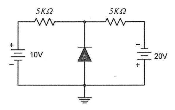
If the diode is Germanium-based, what is the current flown through the diode?
