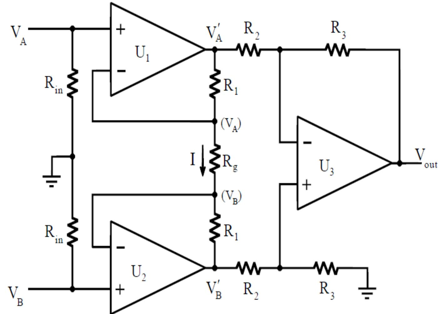
$$V_{out} = \frac{R_3}{R_2} (V'_B - V'_A)$$
